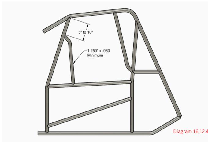
x) **Chassis Front Upright Support Bars: In 2026, the use of extended front upright support bars added to chassis is highly recommended. This will most likely be mandatory in 2027 after input and study to finalize specifications. For reference, the dimensions in diagram 16.12.4 are proposed dimensions and are not final at this time.**
