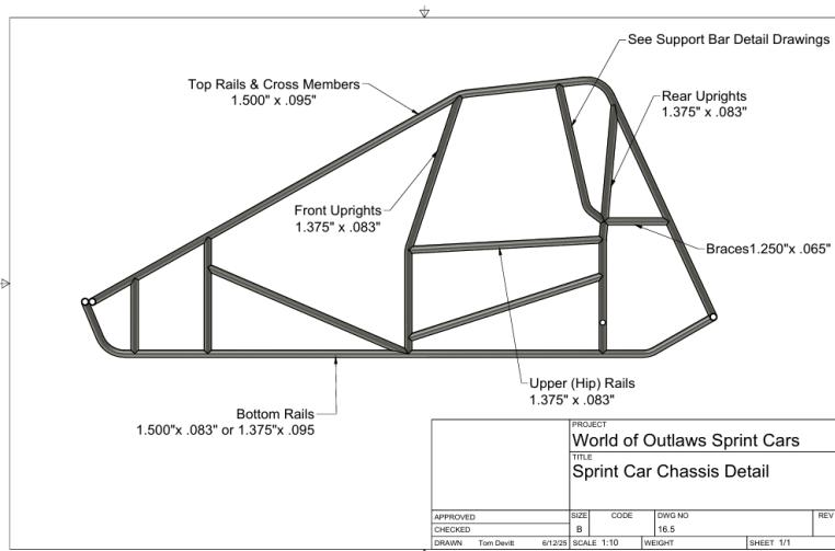
y) Chassis Support Bars: All chassis are required to have additional bars installed to support and decrease the span between the front and rear uprights in the driver's area. The support bars must be in addition to the front and rear uprights. Any attempts to manipulate the front and rear uprights to conform to these measurements will not be allowed at the discretion of Williams Grove Speedway officials.
